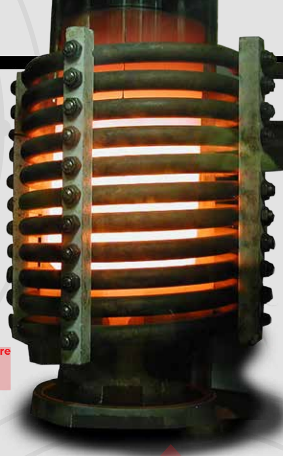
Plutonium is heated by coils at PF-4.
