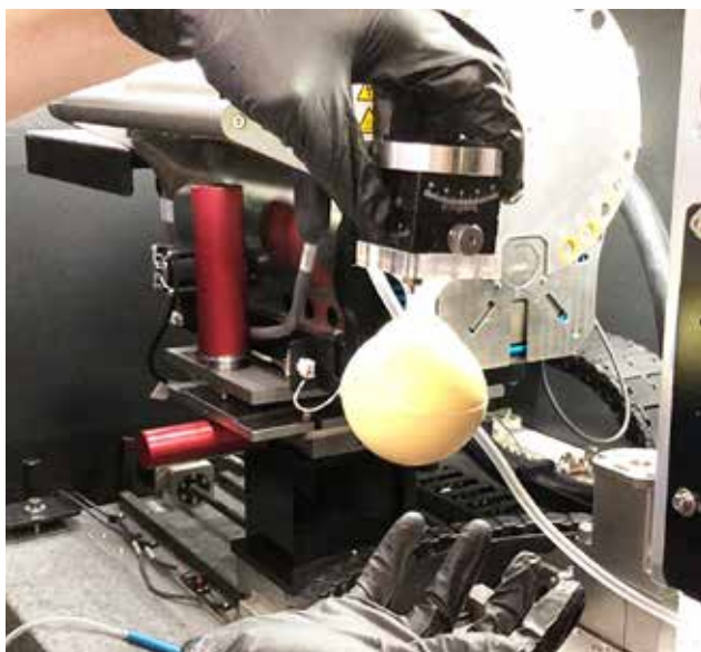
▲ One air-buoyant solid prototype clung to its vacuum chuck for more than a minute, supported by nothing more than ambient air pressure.
