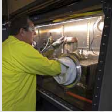
A worker uses a glove box to safely handle nuclear materials for the ARIES program.
